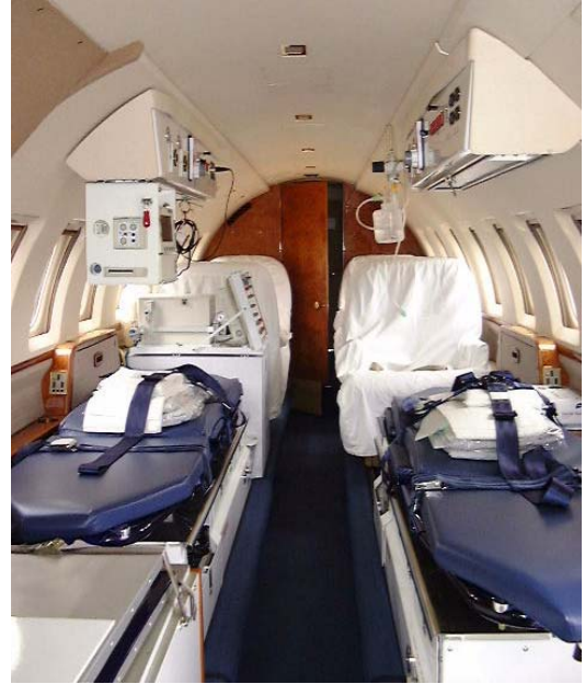
Dual Dedicated System Install
