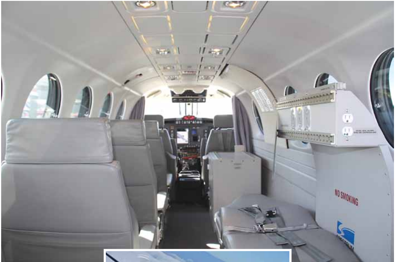
CLOSE-UP: INTERIOR VIEW OF THE SPECIAL MISSION KING AIR 350ER SHOWN WITH MEDEVAC AND HIGH DENSITY SEATING; (INSET) IN FLIGHT
