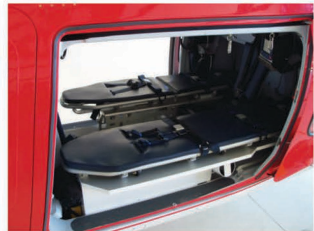
Main Base and Stretcher and Secondary Base and Stretcher Installed with Medical Attendant Seat
