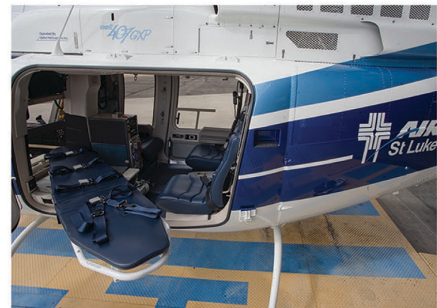
Stretcher on pivot – sliding into aircraft
